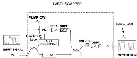
**Figure 2.** Schematic representation of the FOPA-based AOLS technique. HNL-DSF: Highly Non-Linear Dispersion Shifted Fiber, A: Attenuator.
