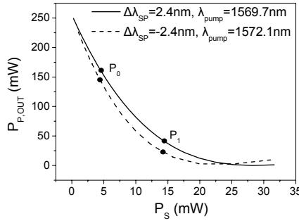
**Figure 7.** Power characteristics of the even-numbered (solid line) and odd-numbered (dashed-line) nodes of the transmission system. The dots indicate the points where the average mark and space of the input signal are adjusted for the preservation of the 5dB extinction ratio.
