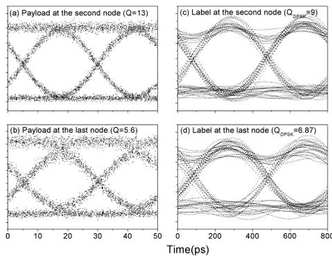
**Figure 9.** *Eye diagrams of both payload and label at the receiver side of the second (a), (b) and the last node (c), (d).*
