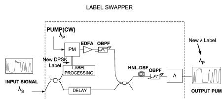
**Figure 2.** Schematic representation of the FOPA-based AOLS technique. HNL-DSF: Highly Non-Linear Dispersion Shifted Fiber, A: Attenuator.
