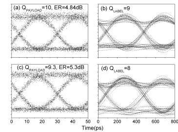
**Figure 6.** Eye diagrams and  $Q$ -factor values of the input (a), (b) and output (c), (d)  $40\text{Gb/s}$  payload and  $2.5\text{Gb/s}$  label data.
