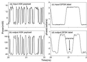
**Figure 5.** The amplitude and phase characteristics of the input (a), (c) and the output (b), (d) packet. In the parametric process, the input packet corresponds to the signal and the output packet appears in the depleted pump.
