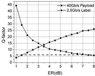
**Figure 3.** *Q-factor calculated for both payload and label in terms of the payload extinction ratio*
