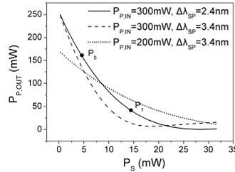
**Figure 4.** *Pump power  $PP,OUT$  at the output of the FOPA in terms of the input signal power  $PS$  for two signal-pump wavelength spacings  $\Delta\lambda_{SP}=\lambda_S-\lambda_P$*
