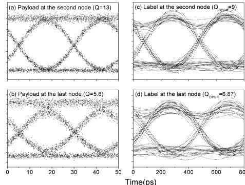
**Figure 9.** *Eye diagrams of both payload and label at the receiver side of the second (a), (b) and the last node (c), (d).*
