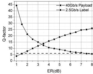
**Figure 3.** *Q-factor calculated for both payload and label in terms of the payload extinction ratio*
