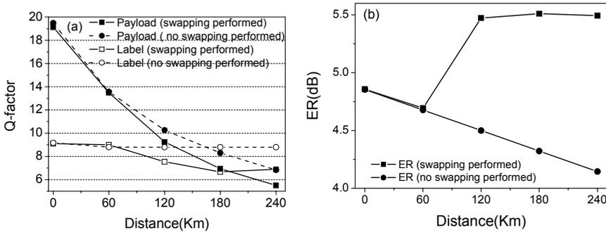
**Figure 8.** *Q-factor performance for both payload and label (a) and the payload extinction ratio (b) in terms of transmission distance. The squares correspond to the case that the intermediate nodes perform swapping, while the circles correspond to the case that no processing is applied at the intermediate stages.*
