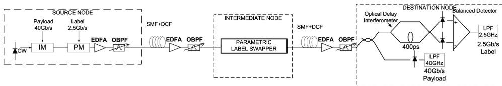
**Figure 1.** Schematic representation of a network consisting of nodes performing parametric label swapping. IM: Intensity Modulator, PM: Phase Modulator, EDFA: Erbium Doped Fiber Amplifier, OBPF: Optical BandPass Filter, SMF: Single Mode Fiber, DCF: Dispersion Compensating Fiber, LPF: Low Pass Filter
