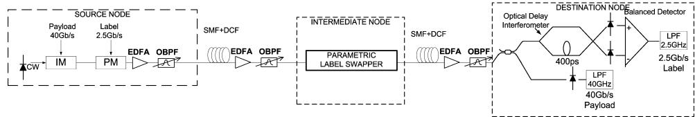
**Figure 1.** Schematic representation of a network consisting of nodes performing parametric label swapping. IM: Intensity Modulator, PM: Phase Modulator, EDFA: Erbium Doped Fiber Amplifier, OBPF: Optical BandPass Filter, SMF: Single Mode Fiber, DCF: Dispersion Compensating Fiber, LPF: Low Pass Filter
