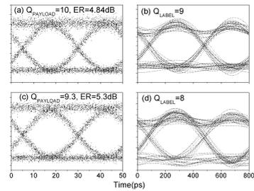
**Figure 6.** Eye diagrams and  $Q$ -factor characteristics of the input (a), (b) and output (c), (d) 40Gb/s payload and 2.5Gb/s label data.
